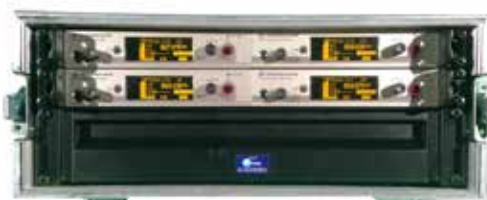
Rack HF - 4x Sennheiser EW300 G3
